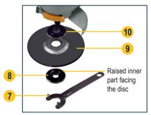
Depressed disc (4 mm or less in thickness)
